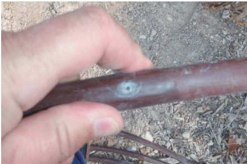
Photo 52. Drip tubing showing the opening of an embedded drip emitter for the release of a precise amount of water in Lph or gph (photo by R. L. Morris)
