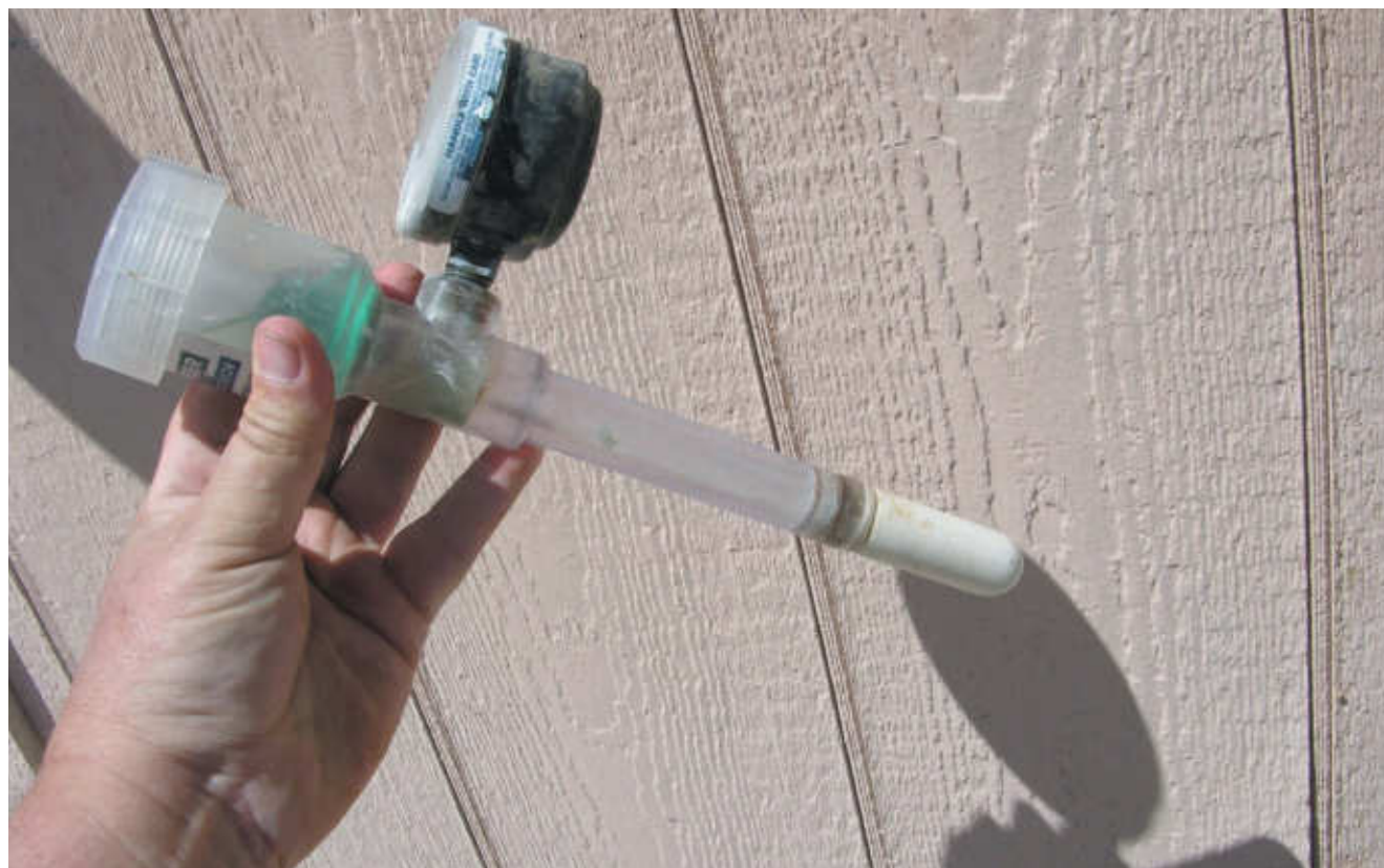
Photo 57. A tensiometer is an instrument filled with water that is placed in direct contact with the moisture in the soil via a ceramic tip. Soil moisture is indirectly assessed as a vacuum (negative pressure) created on the tensiometer's internal water, which is recorded with a gauge. It is used for assessing when to schedule irrigations. (Photo by R. L. Morris.)
